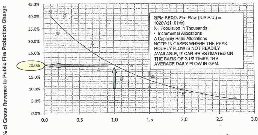
Ratio = PEAK HOUR RATE GPM / REQD. FIRE FLOW (N.B.F.U.)\* GPM
