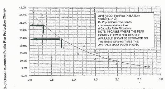
Ratio = PEAK HOUR RATE GPM / REQD. FIRE FLOW (N.B.F.U.)\* GPM
